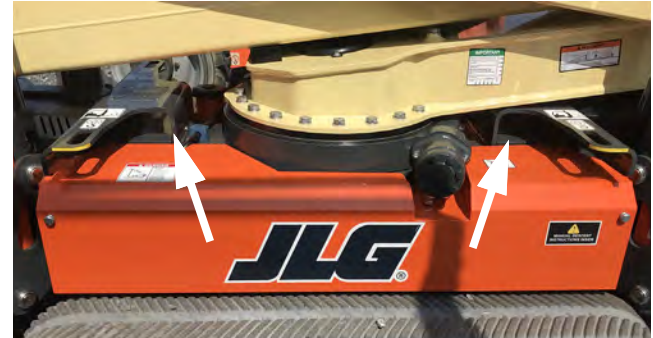
Figure 4-7. Lifting Machine - Fork Lift Pockets Location
