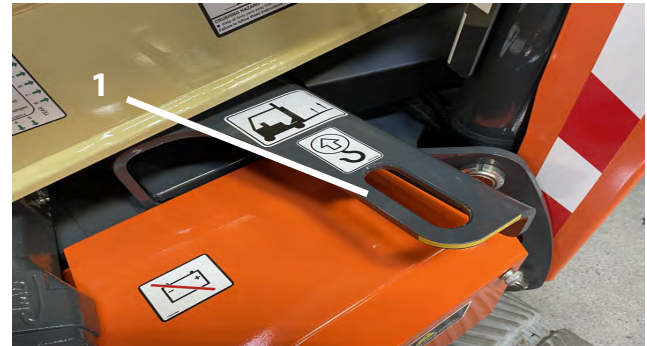
Figure 4-5. Lifting Machine - Lifting Lugs Location
